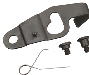
Short-stop Latch protects wire strands by limiting the stripping stroke to \frac{9}{32} in. and retains the slug until the wire is ready for terminating.
