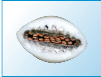
Diagonal cutters do not cut cleanly and decreases the quality of the strip.
